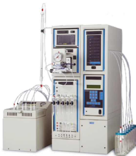
PowerPrep GPC /Sequential system processes 5 samples sequentially
