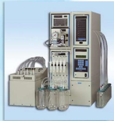
The Power-Prep SPE automated One Step Extraction and Concentration System is built by design to simplify, improve and increase your productivity by automating the manual steps in your sample preparation process. Automating time consuming steps involved in sample extraction and concentration lowers your labor, solvent consumption and disposal costs as much as 90%.
